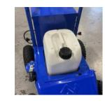
3. Pour water into 30L tank, then add your desired ratio of paint and stir thoroughly, ensuring all paint and water is mixed.
