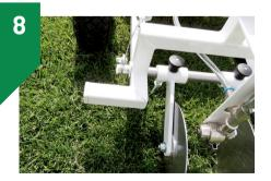
Feed the cable through the hole in the cable clamp bolt and tighten it.
