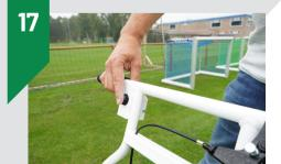
Switch on the machine and rinse until paint comes out.
