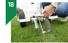
As soon as paint comes out, return the ball valve to horizontal postition.
