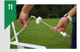
Connect the tube to the suction rod.
