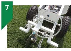
Feed the cable through the holes provided in the chassis.
