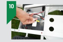
Attach the yellow plug to the battery. Replace the lid and secure using supplied bolts and allen key.
