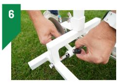
Set the discs to the desired width of the line.
