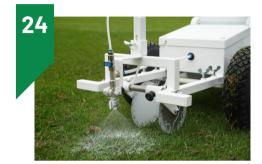
Return ball valve to horizontal position to rinse spray head and nozzle.
