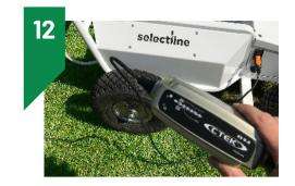
Connect the charging plug to the machine and the charger to a 220V socket. An indicator light tells you the charge level. The battery is fully charged when the '5' lights up green.
