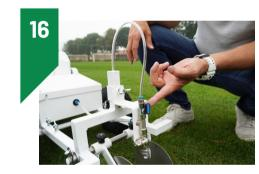
Turn the ball valve to vertical position.
