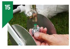
Put the nozzle in the nozzle holder, place the flat seal firmly on top of it and finally the filter. Then screw the nozzle holder onto the spray head.
