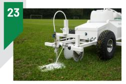
Turn the ball valve to vertical position and rinse the tubes by pressing the
